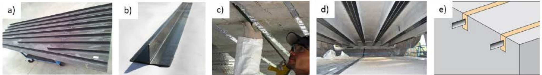
Figure 1. Example of the COM2BUILD approach: composite components from aircrafts, a), can be easily sliced in flat patches, bars or T-shapes, b), then reused for the repair of buildings as external reinforcement, d), or near-surface-mounted, c) and e).
