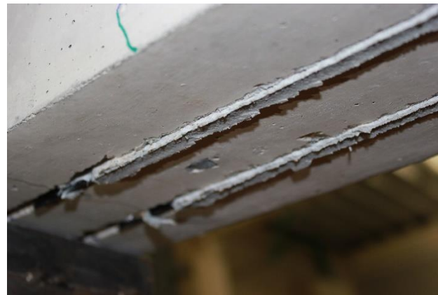
End-debonding at 70 °C
