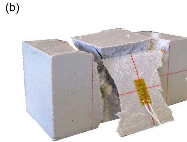
Compressive failure mode
