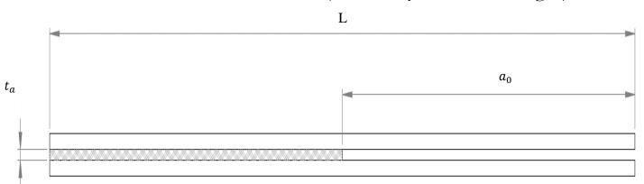
L x W x H = 200 x 25 x 3 mm  $t_a = 0.4 - 0.7$  mm  $a_0 = 100$  mm Pre-crack = 10-15 mm
