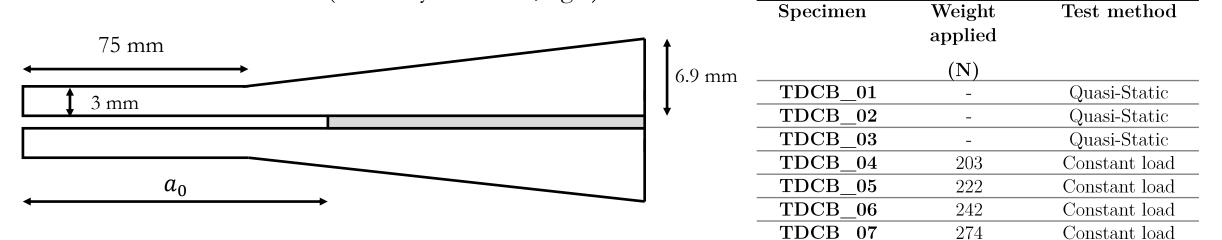
L x W = 200 x 25 mm  $t_a$  = 0.6 - 0.9 mm  $a_0$  = 100 mm Pre-crack = 10-15 mm
