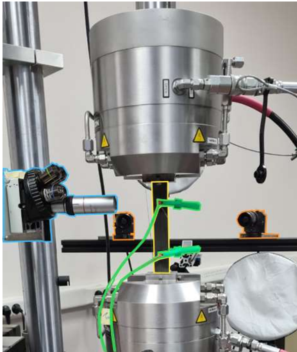
Tensile test experimental set up on the IMA/M21ev
